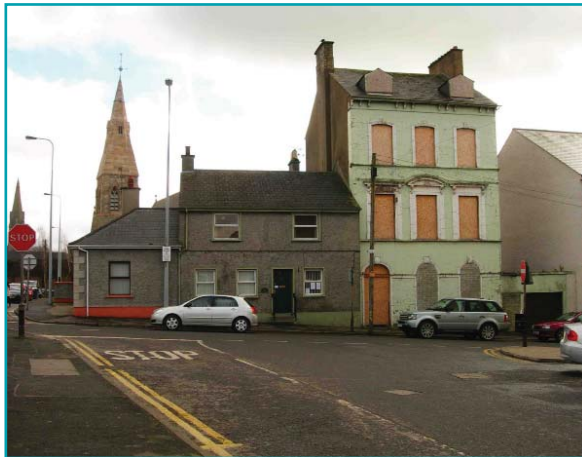
Patrick/Church junction (top) Excessive width of carriageway makes pedestrian crossing more hazardous, increases vehicle turning speeds, and is unsightly.
