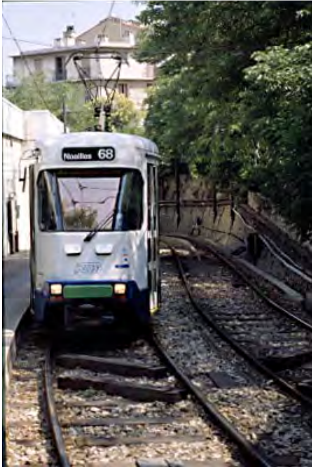
The existing tramway in Marseille. Note the narrow vehicle gauge. Photo: Bertil Hylén, VTI.
