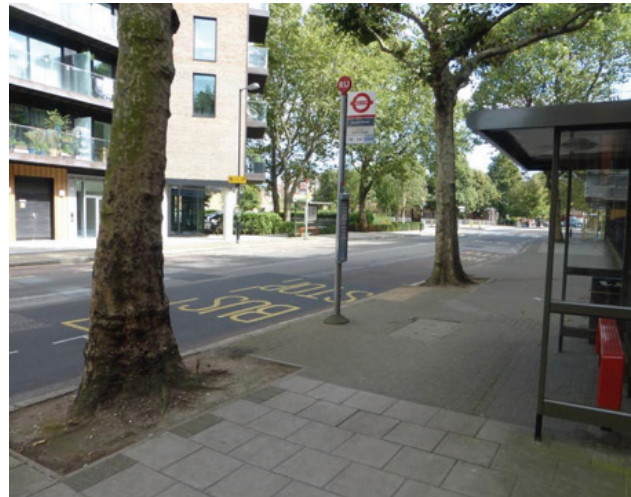
Figure 32: Pair of bus stops serving higher-density development, well overlooked, and with good intervisibility (Walworth, London). The stop on the far side is integrated with a 'pocket park'. (Photo: Tim Pharoah, 2017)
