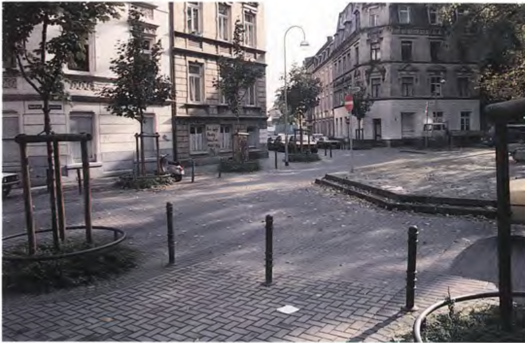
18: Paving details in the Nippes district now reflect the geometry of buildings rather than the geometry of traffic. Here part of the street has been raised, forming a "stage" at the entrance to a church.
