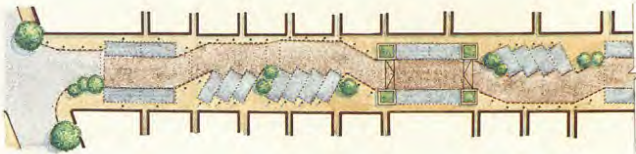
29: Lateral shift in the carriageway formed by angled parking bays defined with planting and cast iron bollards. (Photo: Leicester City Council)
