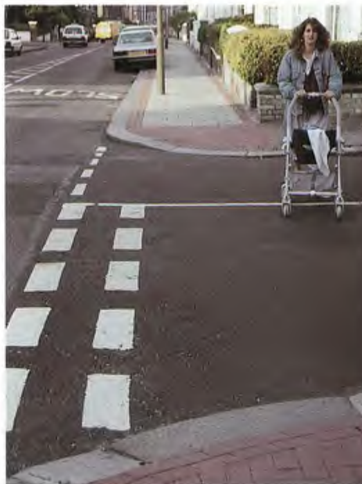
14: Excessive corner radii encourage speeding and are hazardous for pedestrians. (Photo: T. Pharoah)
