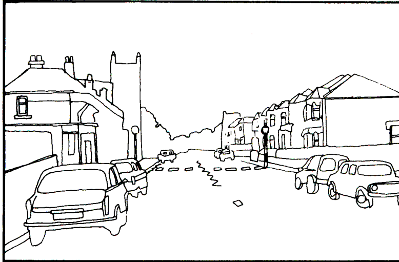
FIG. 21 ZEBRA CROSSING WIDTH REDUCED BY FOOTWAY WIDENING (Fulham) Note that the footway has been widened only at the crossing itself. It is better to widen across the entire section covered by the "zig-zag" markings.
