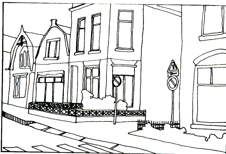
FIG. 14 RAISED FOOTWAY ACCROSS MOUTH OF JUNCTION (Hoorn, Holland)
