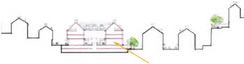
Section AB through new mixed-use buildings Residential and office space over shopping at street level
