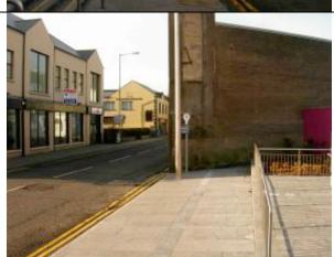
After Dock Street the footway begins again. It is of reasonable width, but this is reduced by the lamp posts that are located twice the required distance from the kerb.
