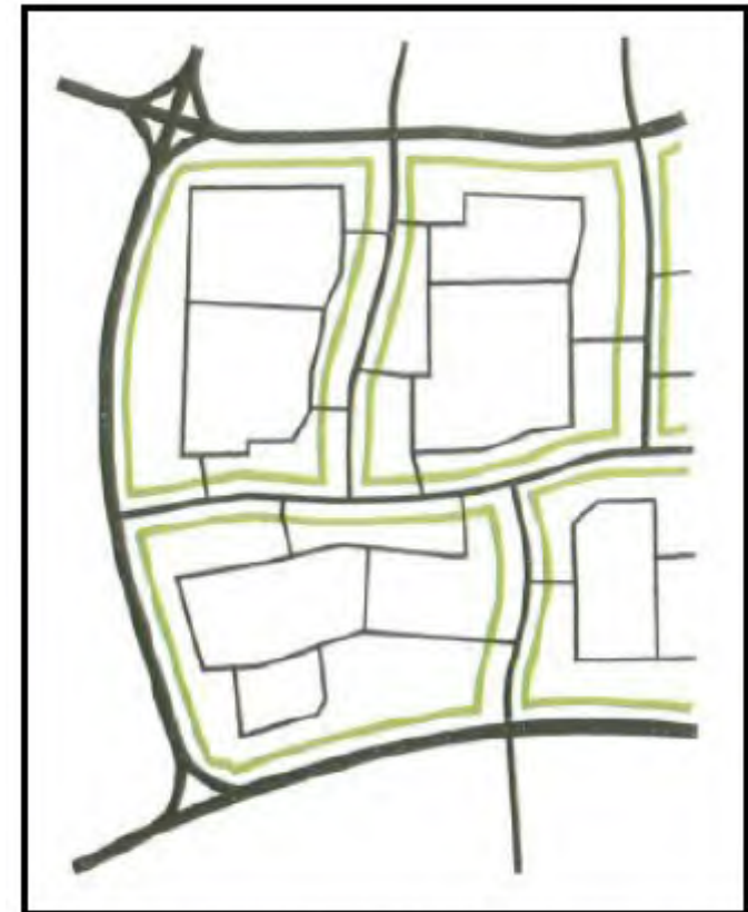
The principle of the hierarchy of distributors. Access roads not shown.
